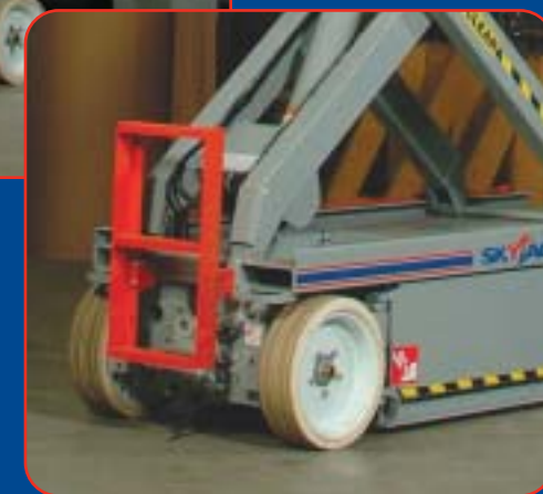
SJIII Conventionals feature variable speed rear wheel hydraulic drive.
